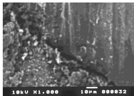
Fig. N121: Interface cemento TopSeal-Diente
