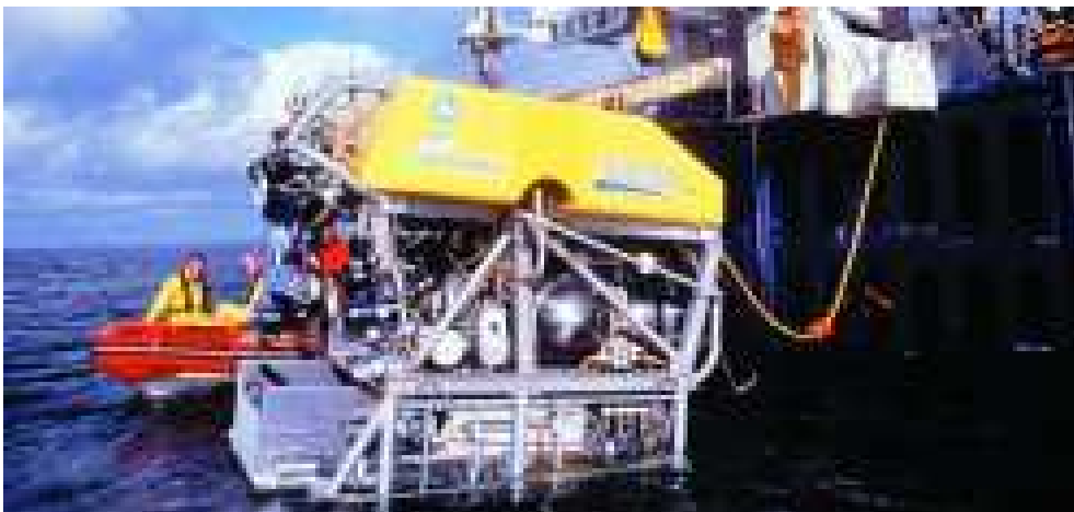
Figura 1.18: Robot submarino Víctor 6000 (IFREMER)
