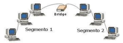
Figura 2. 7: Bridge enlazando red
