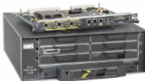
Figure 1. The Cisco 7200 VXR Router Series with Network Processing Engine NPE-G2
