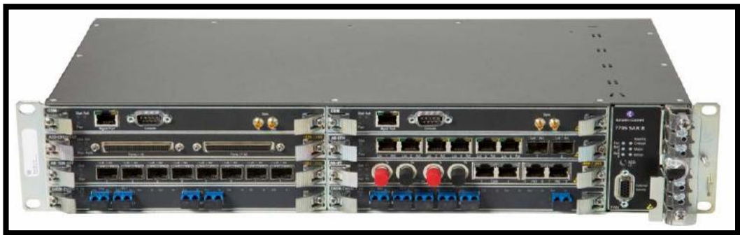
Figura 3. 5: Router 7705 SAR-8 Fuente: (ALCATEL-LUCENT UNIVERSITY, 2012)
