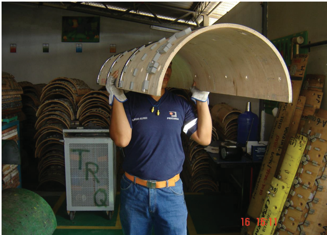
Picture 5: Machine Operator carrying a wooden ward blueprint for the die cutter
