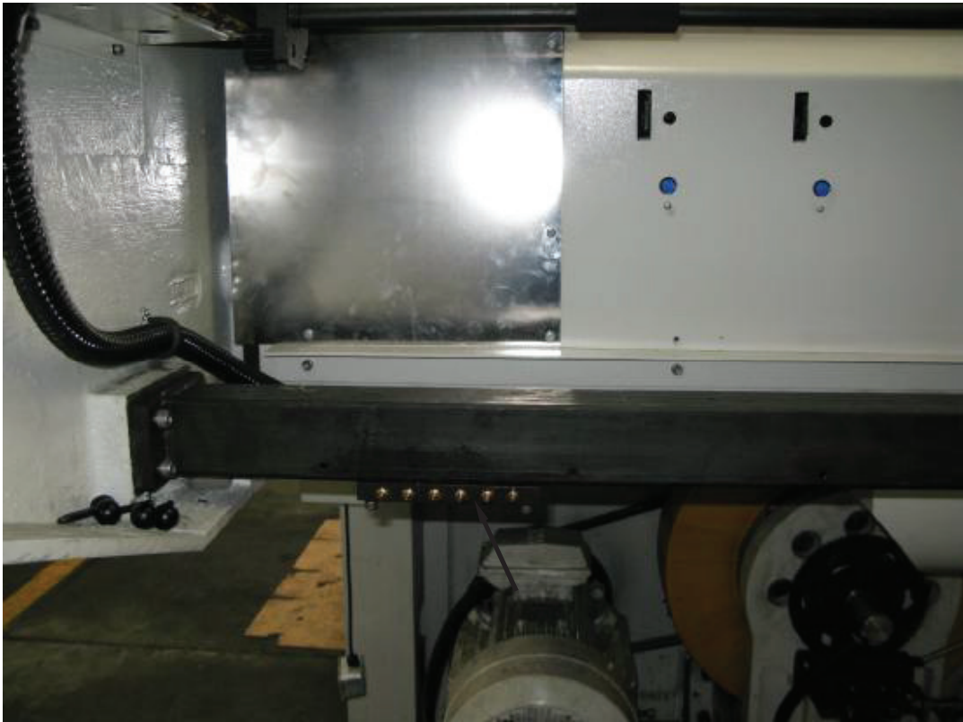
Figure 1. Front conveyor drive lubrication cream nozzle (symmetrical), filling type: A
