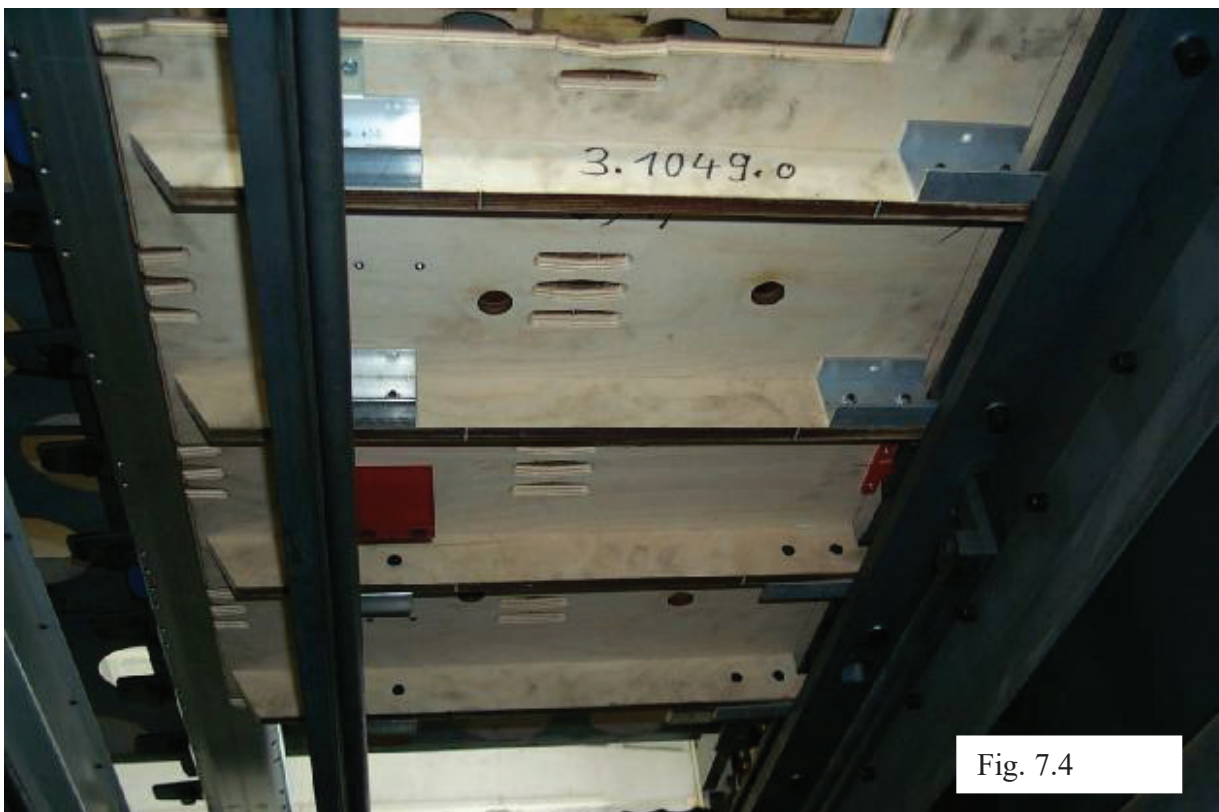
Fitting of female stripping board
