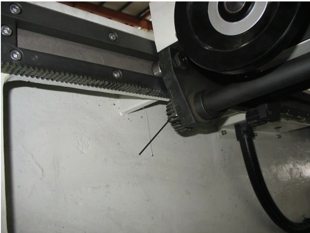
Figure 2. Moveable support rack (symmetrical), oil filling type: A
