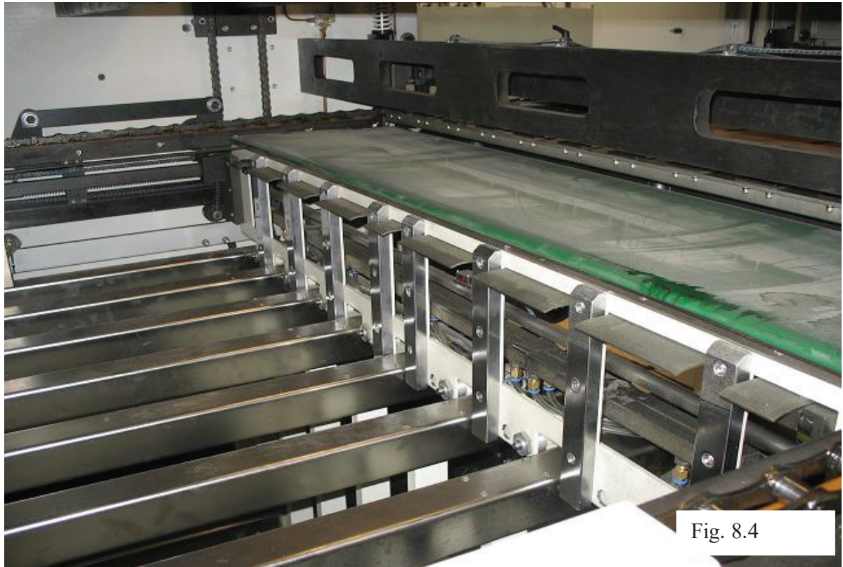
Pulling the upper tool carrier crossbar out.
