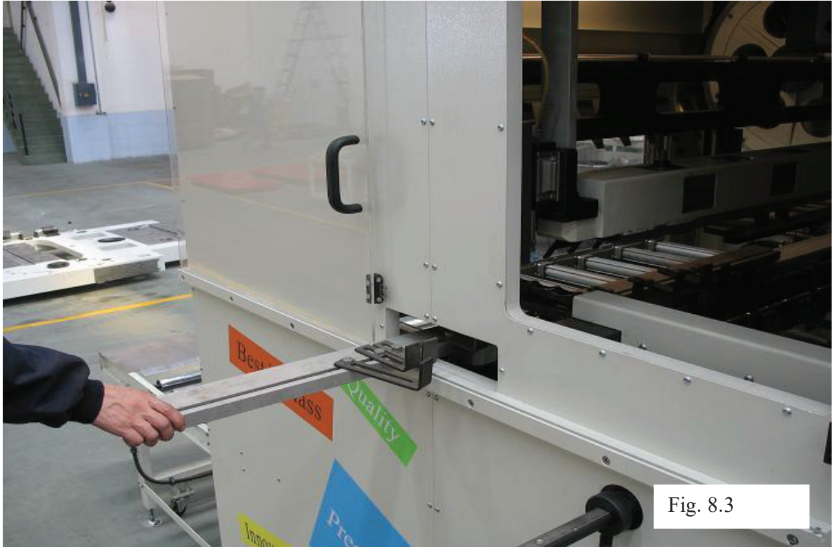
Pulling the upper tool carrier crossbar out.
