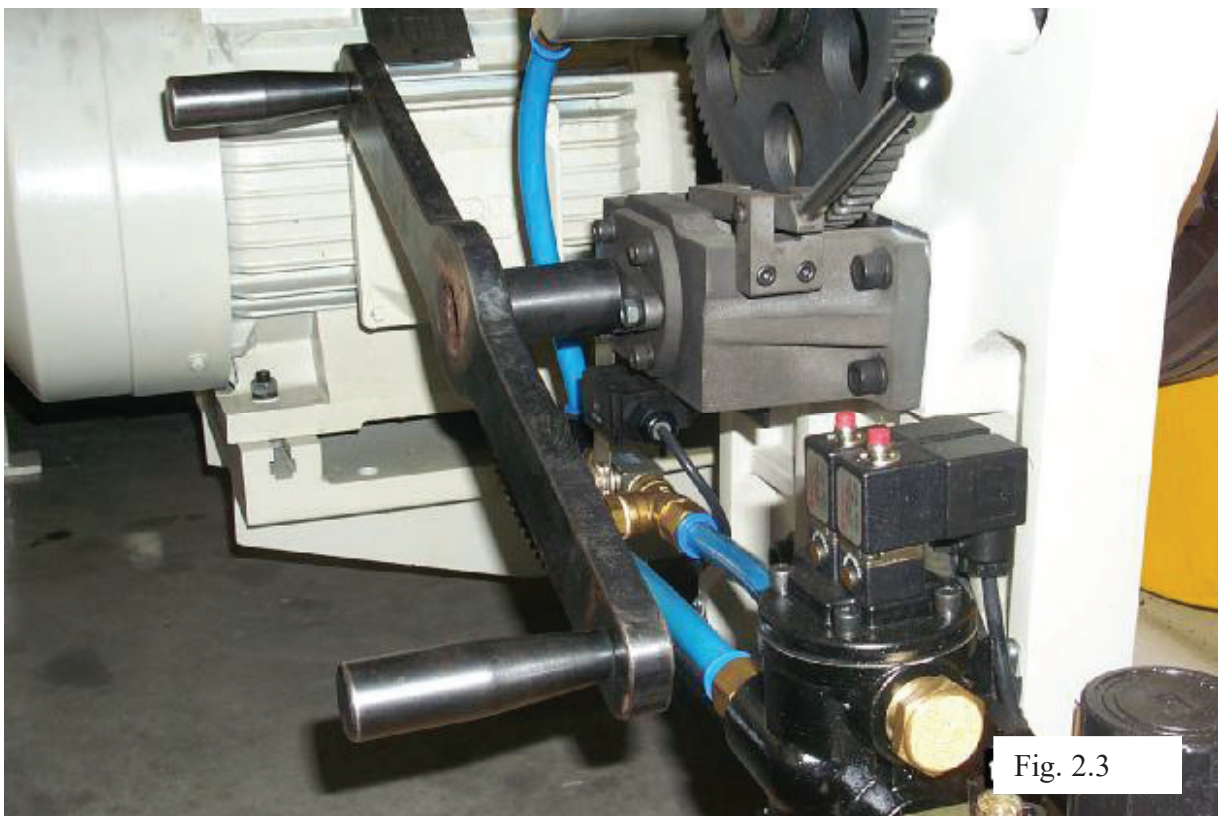
Insert and push in the ratchet wrench at the end of the shaft.
