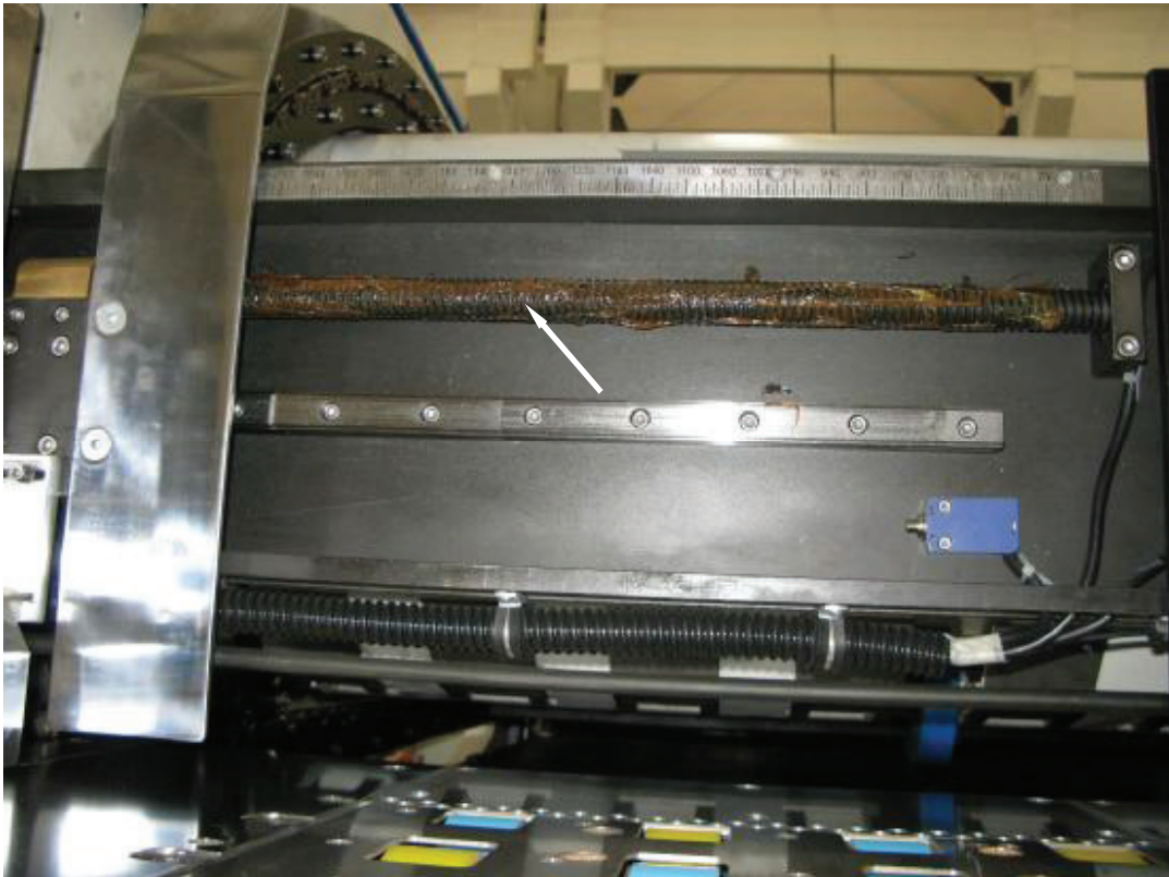
Figure 4. Side guide screw rod (symmetrical), oil filling type: A
