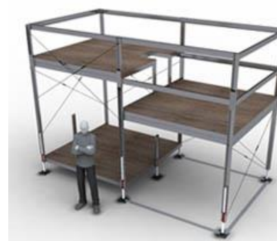
2 assemble frame and floors
