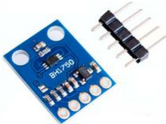
Figura 7. Sensor BH1750 (ROHM SemiConductor, 2009)
