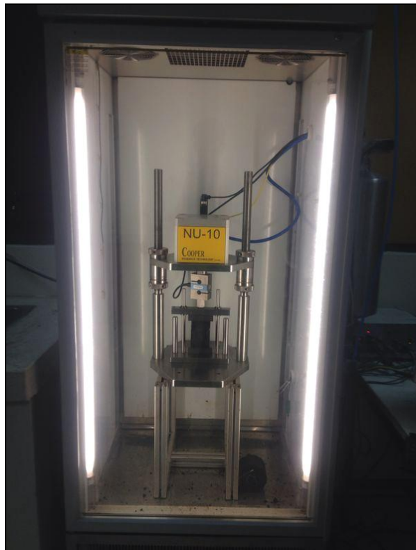
Figura 24: Nottingham Asphalt Tester (NAT).
