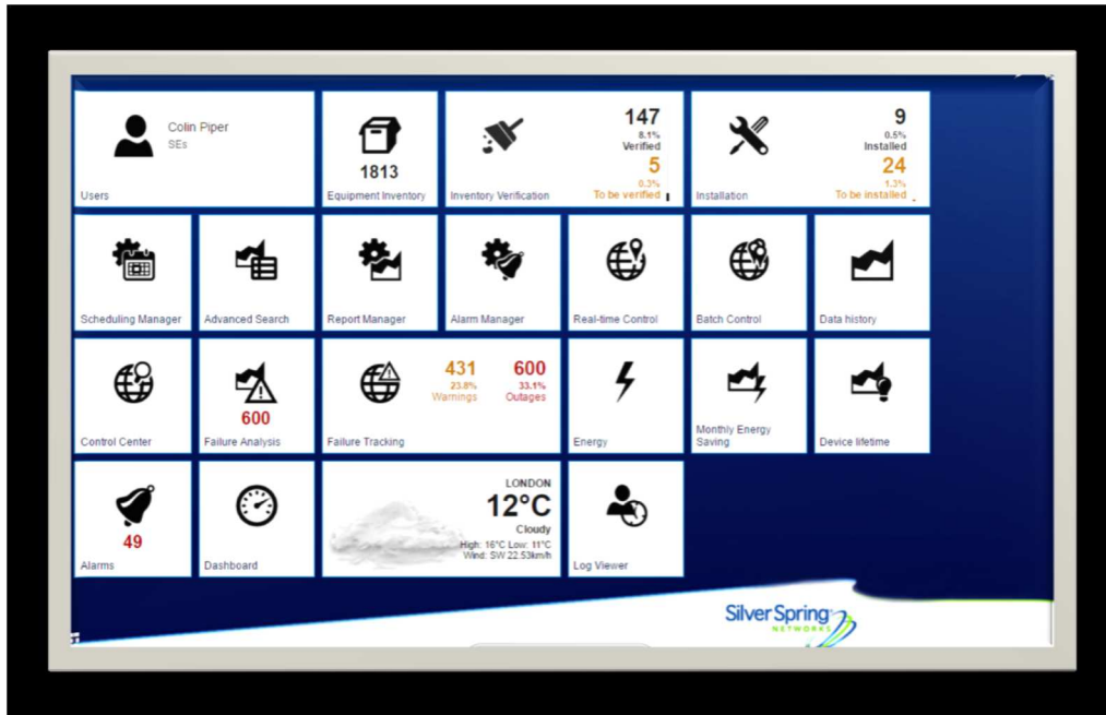
Figura 4.2: STREETLIGHT.VISION USER INTERFACE Fuente: (Aldis, 2018)
