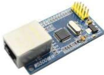
Figura 3. 8: Módulo Ethernet W5500.
