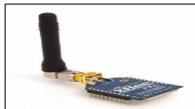
Figura 2.39. Antena 2dBi / 5dBi
