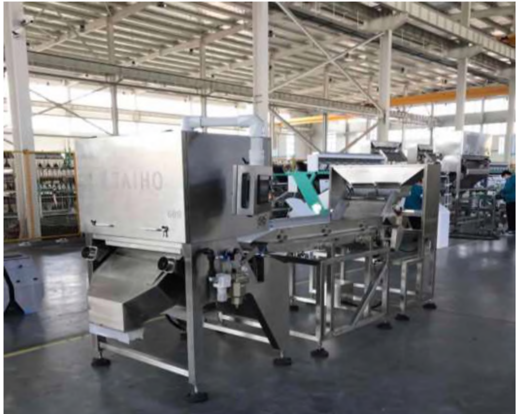
Figura 30 Maquinarias 6SXL-1200 Single-layer-belt-tye color sorter. Tomado de: Empresa TAHIO. 2018.
