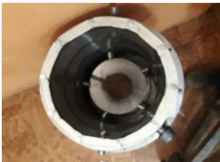
Figura 4. 1 Vista superior del tanque (reactor)
