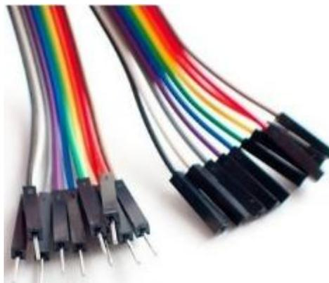
**Figura 35.** *Cables conector Dupont macho y hembra.* Recuperado de <https://ardushop.ro/en/electronics/226-10-x-dupont-wires-male-female-10cm.html>
