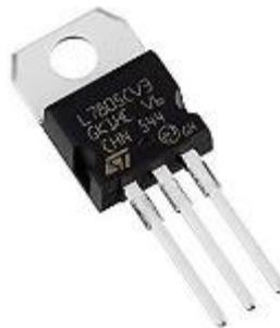
**Figura 22.** *IC 7805.* Recuperado de <https://www.amazon.in/Versatile-7805-5v-voltage-regulator/dp/B00KHK1C6Y>
